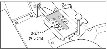
Figure 36. Deck Height Pin Position
